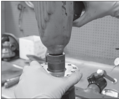
1/2" impact gun on pinion nut setting.
