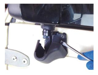
Pop the side view mirror cover open using a standard screwdriver.
