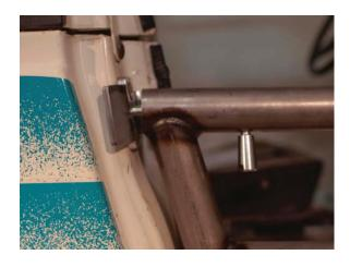
The latch should hit the striker as close to the middle as possible. If it does skip to Step 19. If it does NOT, you will need to loosen the hinge screws and adjust the door up or down and retighten the screws.
