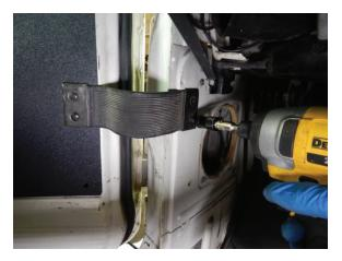
Disconnect the body side of the door strap by removing the (2) phillips screws using a #2 phillips screwdriver. Leave the door strap attached to the door.
