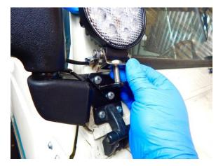
Step 18 Insert the light mounting bolt (or stud) in the light bracket.
