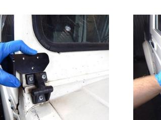
Step 8 Position the supplied passenger side, side view mirror as shown.
