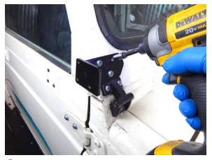
Step 11 Hold the mirror bracket in place and remove all three of the self drilling screws.
