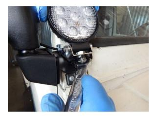
Step 21 Tighten the nut using a 17mm open end wrench.
