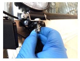
Step 19 Install the supplied lock washer.
