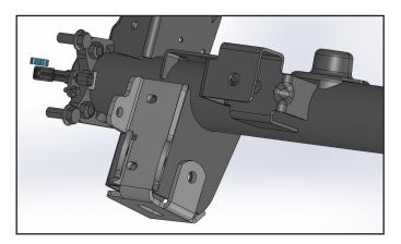
Once the bracket fitment has been verified, remove bracket and coat area with paint.
