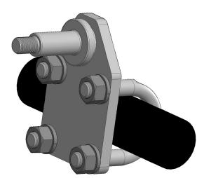
Place the Tie Rod Bracket Assembly (A) on the tie rod in the desired configuration and loosely install the U-Bolt Straps (B) along with the 7/16" Split Lock Washers (C) and 7/16" GR5 Nuts (D). Do not tighten hardware yet.
