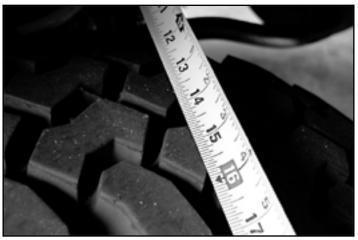
O If the two measurements are equal, the axle is centered. If measurements vary, divide the difference in half to determine the amount of adjustment required. HINT: If axle housing is not centered, the chassis can be laterally shifted using either of the following methods.
