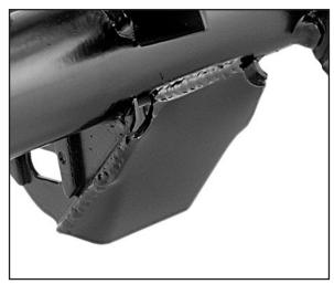
Once all welding is complete, spray paint any bare metal on MiniSkids, suspension arm brackets, and axle tube to prevent corrosion. All exposed metal must be completely covered.
