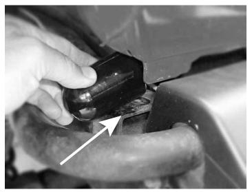
NOTICE: If the factory inverted U-bracket pictured above restricts radiator bumper installation, it must be removed. Remove bracket by cutting from chassis using a suitable cutting tool.
