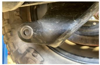
Carefully lower the axle approximately 2 inches, making sure that no other components are binding or being stretched.
