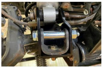
Sleeve 93 will be used in the OE shock mounting position.
