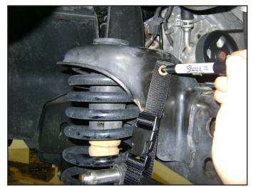
• Attach the lanyards to the drilled hole using the supplied 1/4" hardware.
